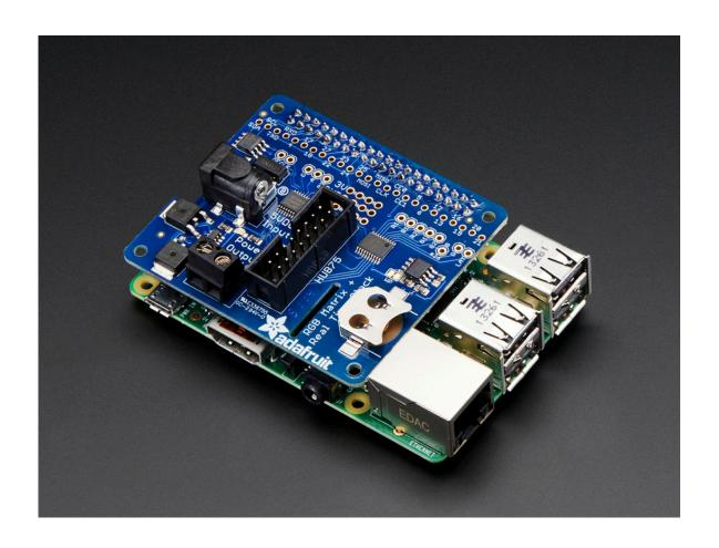
LED GPIO HAT available at Adafruit, it can manage up to 4 32x32 LED Matrix
